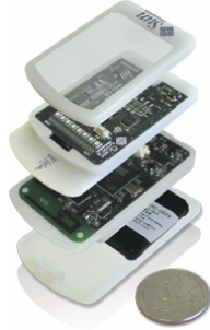
Figure 1. Sun SPOT wireless sensor/actuator device, with a demo sensor board on top, the main processor and radio board in the middle, and a battery board on the bottom.
