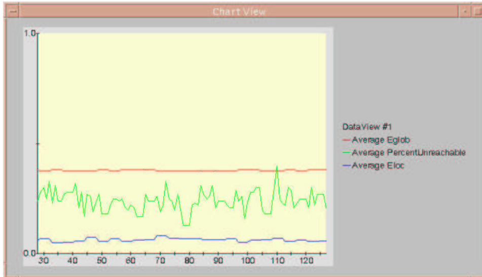
Figure 4: Metrics plotted versus time (rounds). Every peer has 5 friends and N=100 . No peers fail. Keep-alive hop count=3.
