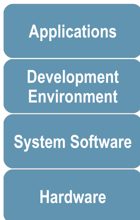
Figure 2: Simple layered model of a computer system
