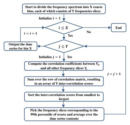
Figure 2. Flowchart of the frequency-binning characterization approach.
