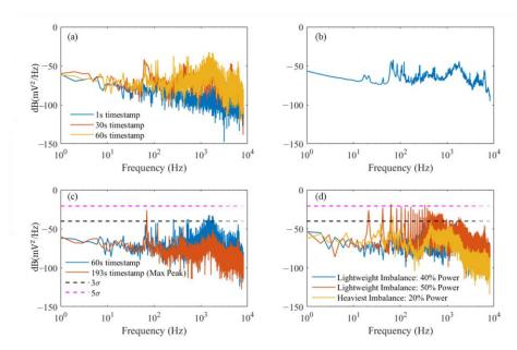
**Figure 7.** The PSD spectrums with frequency thresholds: (a) comparison of healthy state measurements for different timestamps; (b) the entire spectrum; (c) comparison of thresholds and different timestamps for healthy state measurements; and (d) the thresholds comparison with the PSDs of different damaged states.
