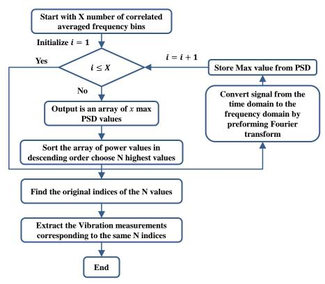
Figure 4. Flowchart detailing the frequency identifier algorithm.
