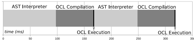
Figure 5: Total time breakdown in seconds of an R application when performing a deoptimization.
