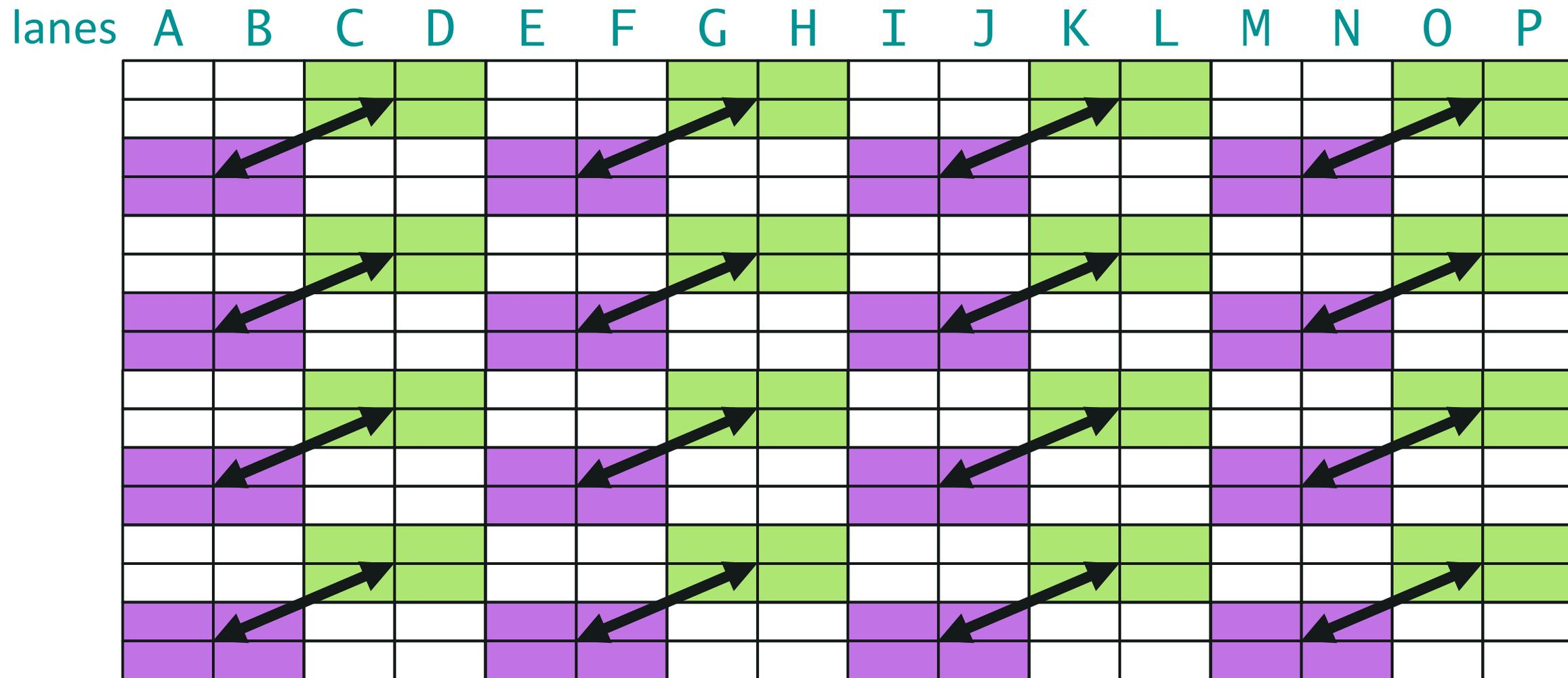
Each column represents the registers used to hold the array **a** for one lane.
