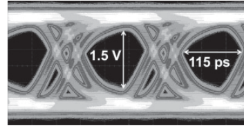
Figure 7: Probed transmitter data eye. Clock skew leads to data-dependent deterministic jitter. Eye shows 2 V modulator drive at 5 Gbps, measured BER was under 10^{-13} and total power under 3 mW.
