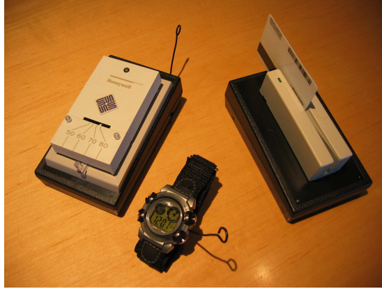
Figure 6: ECC-enabled wireless devices built at Sun Labs: (a) thermostat, (b) health-monitoring watch (c) magnetic stripe reader.
