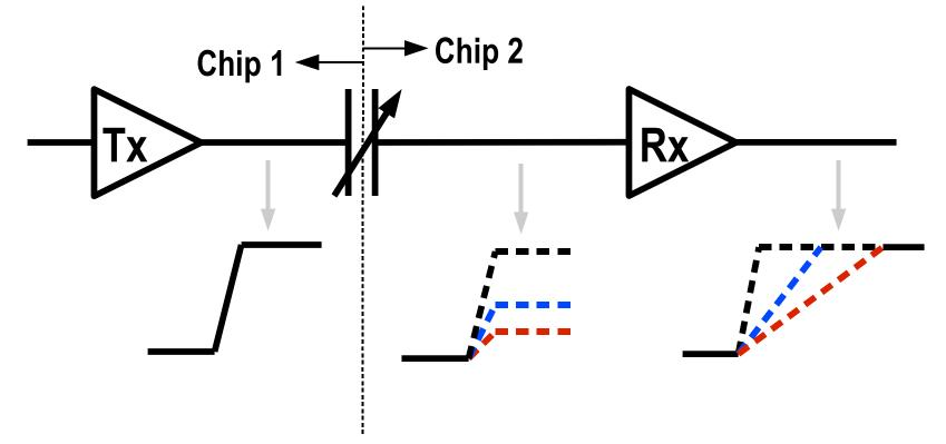
Typical channel delay ~ 5 gate delays
