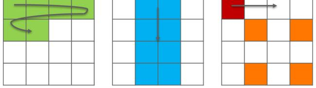
Figure 14: The three types of data access pattern in the disparity computer vision workload.
