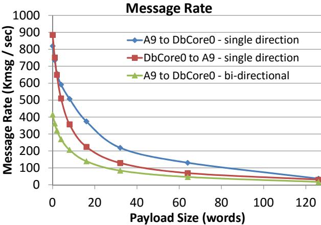
Figure 10: Mailbox throughput as a function of payload size
