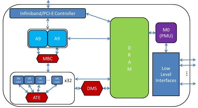
Figure 1: Block diagram of a DPU
