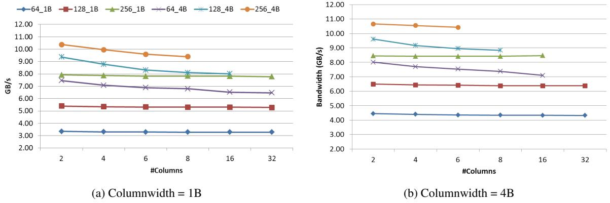
Figure 6: Bandwidth achieved across 32 dbcores for reading (a) and reading and writing(b) data via the DMS. Each line shows the bandwidth achieved for given number of rows per buffer and column width
