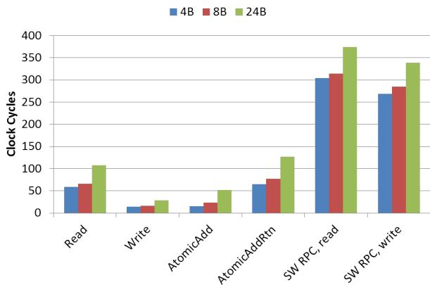
Figure 9: Performance of ATE SW and HW RPCs for different payload sizes
