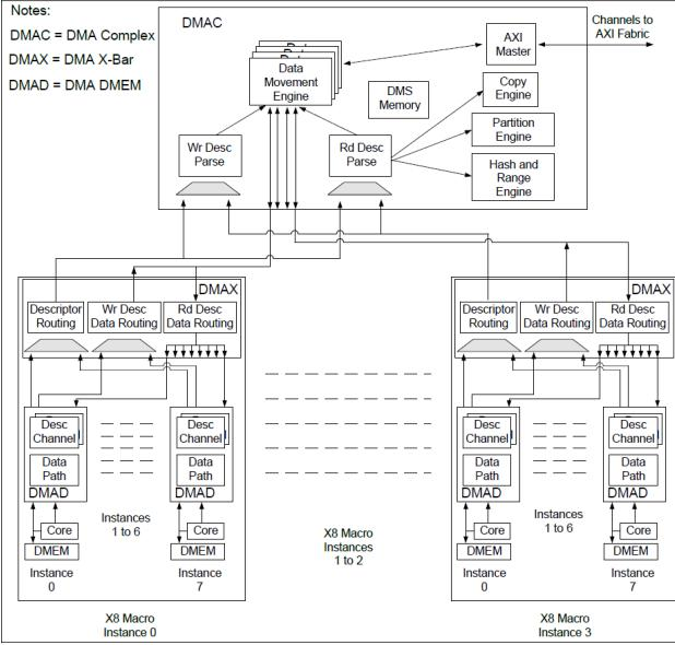
Figure 3: Data Movement System (DMS)
