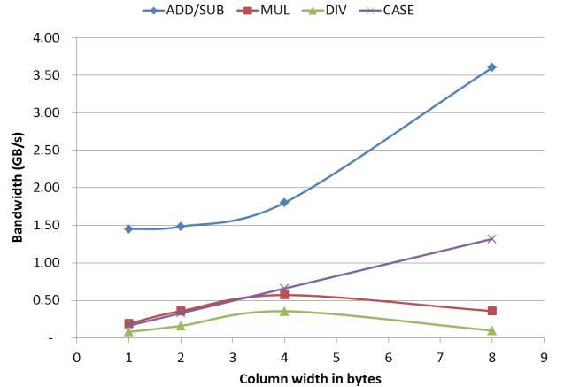
Figure 12: Performance achieved for a single dbCore for the filter primitive
