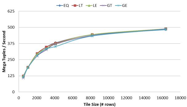
Figure 11: Performance achieved for a single dbCore for the filter primitive
