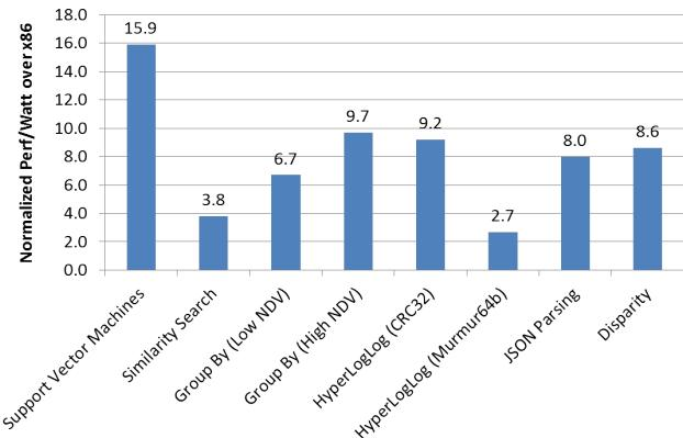
Figure 13: Power efficiency gains of the DPU for several applications
