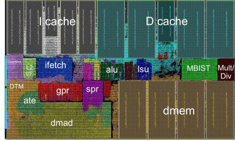
Figure 4: dbCore processor implementation
