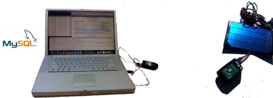
Figure 1: The experimental setup includes a laptop with an attached basestation communicating with a solar-powered Sun SPOT, about 15 feet away, using the 802.15.4 radio. The SPOT is placed outside the window of the office that has the laptop. Sensor data is stored in a mySQL database installed on the laptop.
